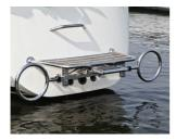
Set the rings vertically. Reverse the dinghy astern of your boat and lift the pontoons into the rings. One side at a time.
